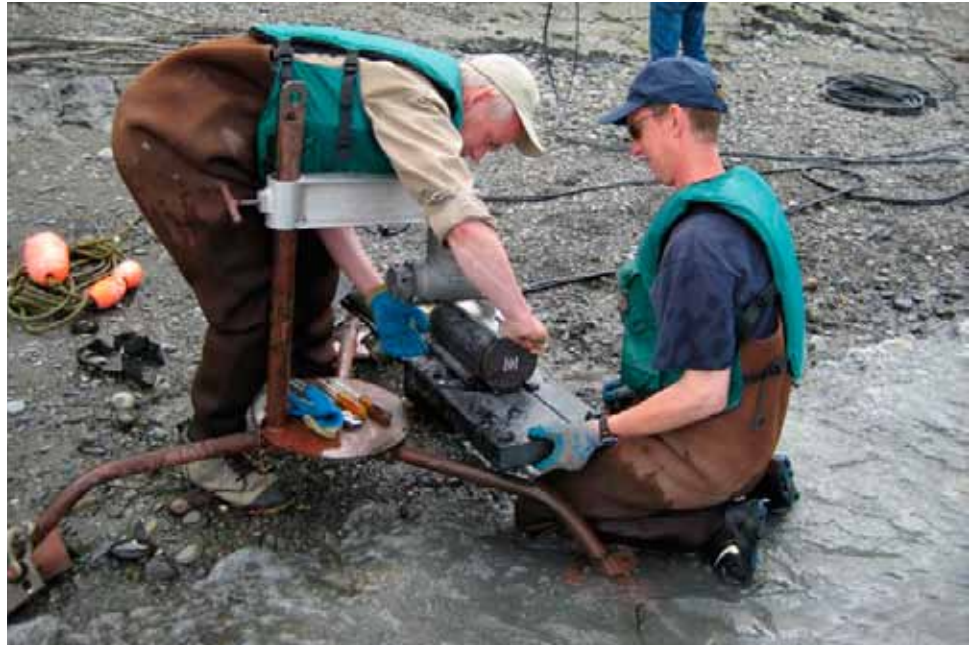
Biologists prepare a DIDSON sonar for deployment in the Kenai River.
