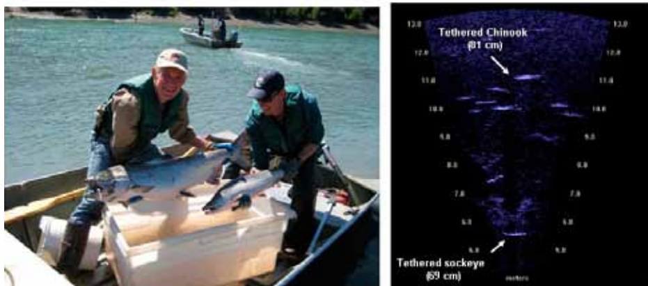
Experiments with tethered fish of known size and species (left) are being conducted to determine whether size information derived from DIDSON images of fish (right) is accurate enough to be used for species classification.
